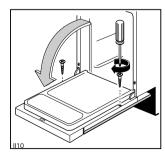
Once the correct position has been found, open the door and fasten the decor panel on the lower section by means of the two long 4x40 screws provided, using the holes through the inner door (see fig.).
